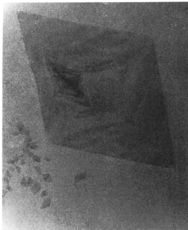
Figure 2. Bright field electron micrograph of a chain-folded monolamellar crystal of n\text{-C}_{168}\text{H}_{338} .
